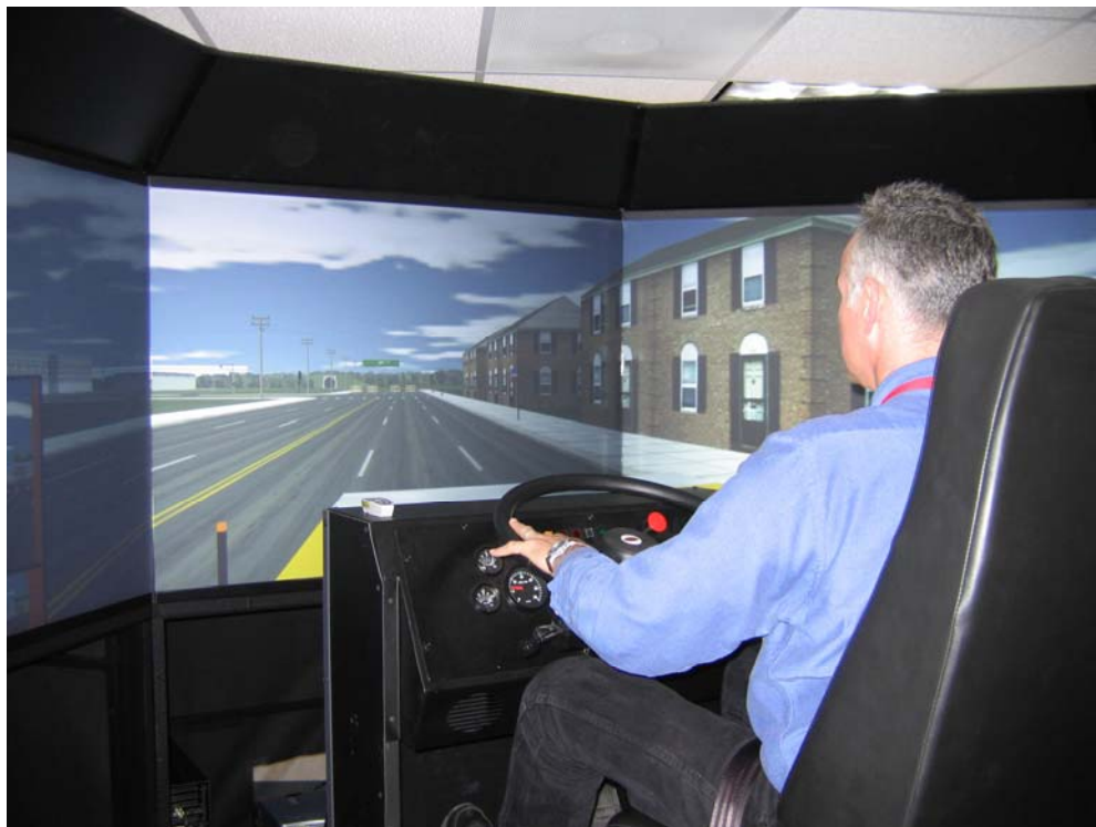
FIGURE 1 “Full mission” truck driver training simulator being employed in the SimVal study.
