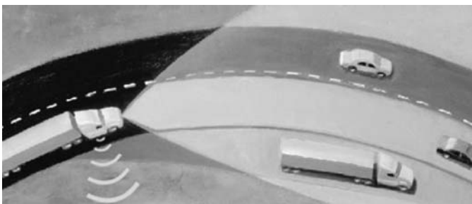
Figure 3. Monopulse lane coverage.
